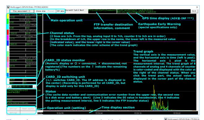
When an alarm occurs, the measured value turns red and the alarm sounds as below. The text (: Alarm) is added next to the measured value. Even if the alarm condition disappears, the red display may continue for several seconds. In addition, only the alarm of the ID of the screen that is currently active (displayed) is activated.
