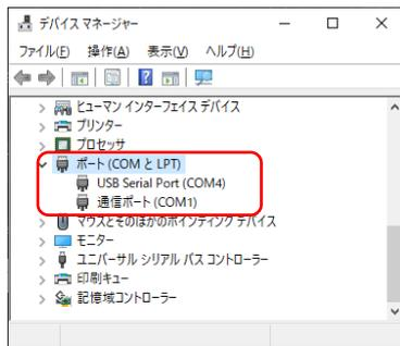
Start the configurator "MultiCardIDConf.EXE" and make settings related to the serial port. Specify the COM number and speed (115.2Kbps or 921.6Kbps) depending on the hardware you are connecting to. The buffer size is default Large (4096). If that doesn't work try Small(14).
