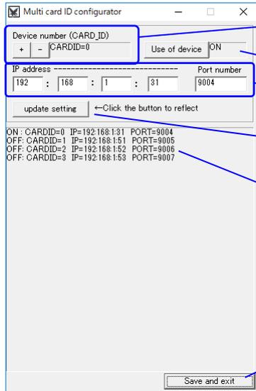
It is CARD\_ID. The unique number assigned to the device is 4-27. The following IP address, port number, and setting of device use are given to this number.
