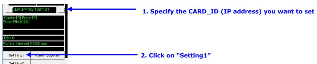
The "Signal adjustment settings" dialog pops up. At first, the button etc. are grayed out and setting is impossible including the edit box part. This can be awakened with a password. Enter "6136" in the top edit box and click the "Adjust lock release" button. Then the gray out of the button is released and it becomes possible to set.
