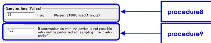
**<Procedure 8: Setting of capture cycle>**
